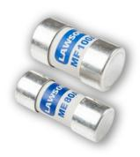
Lawson Type "ME" and "MF" fuse-links are for use in single or three-phase house service cut-outs or similar installations. The standardized BS 1361 breaking capacity of these fuse-links is 33kA at 0.3p.f.
