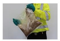
6. Before mixing rotate and shake at the corners to free the powder.
