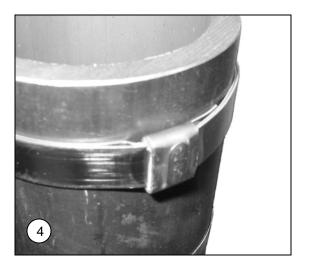
Clamp is now locked and completed. Band will be bent upward 90° and have a cut-off edge that is flush or slightly higher than the buckle.
