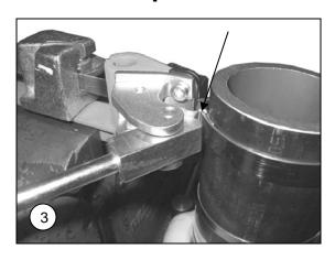
When properly tensioned, roll tool over hose, backing off tension handle ¼ to ½ turn only, through course of rollover, (depending on type and size of hose) until shear hook grips buckle edge. Push cutter handle forward in a quick motion to shear band, completing BAND-IT JR. Clamp.
