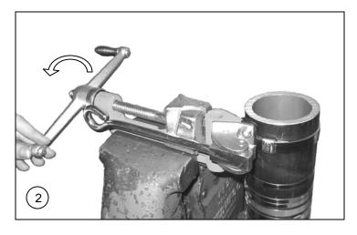
Install clamp over hose assembly. Tension clamp by turning the handle of BAND-IT Tool clockwise. To feel movement of band, place finger on BAND-IT BAND at buckle edge while tensioning with tool handle. When you no longer feel band moving through buckle, MAXIMUM PRESSURE HAS BEEN EXERTED BY BAND-IT BAND.
