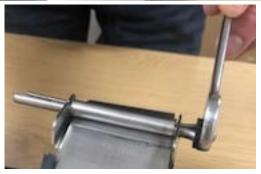
5. Tighten cleat by spinning pin and folding steel. Tighten using brass winding nut and ratchet/spanner. Do not overtighten.
