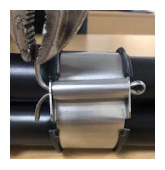
7. Use mole grips to splay end of pin out stopping pin from turning.
