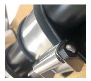
3. Place split pin through **slot hole**, until pin is equal lengths on both sides with end of steel in between pin.
