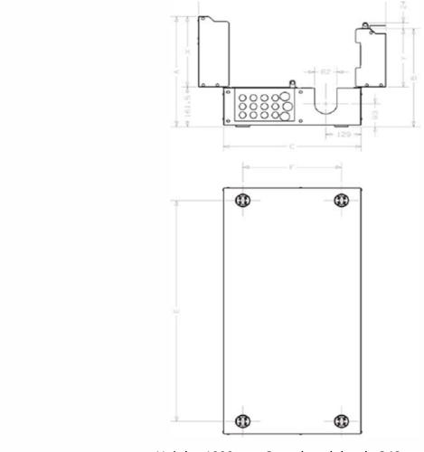
Height: 1000mm, Case closed depth: 248mm
