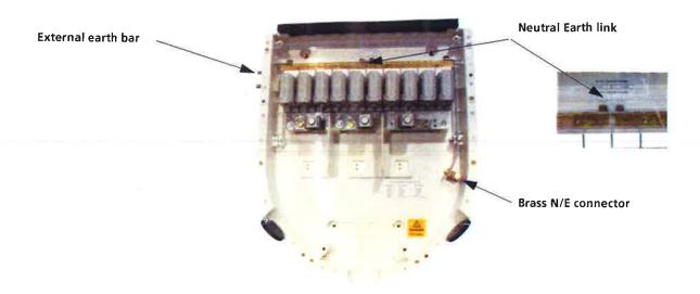
2. Insert the M8 nut in the position indicated. Install the supplementary earth riser bar supplied in the locations in the base of the unit such that it is in contact with the main earth terminal. Loosely tighten the M8 setscrew with its washers up against the riser. Reposition the replacement external earth bar and affix to main earth terminal with the M10 setscrew passing through the earth riser bar (torque setting 20Nm). Final tighten the M8 setscrew.
