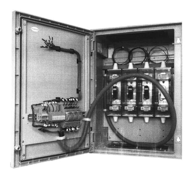
Description: It is a GRP Enclosure 745mm x 535mm x 300mm deep. The meter and CTs are not included. The backplate including equipment and the mounting plate including the terminal rail are packaged separately from the GRP box. This is to overcome the overall weight and so that the box can be mounted and the plates fitted after.
